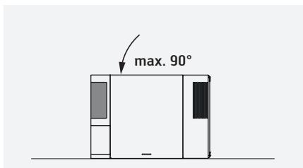
After each transport, the appliance must be left idle for 10 minutes before it may be switched on.
