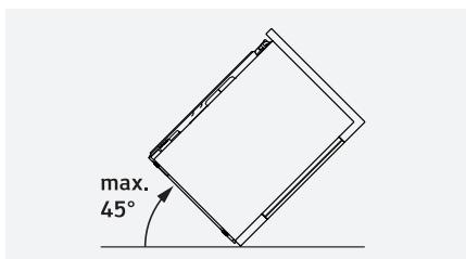
The machine may be carefully laid onto the left side:
